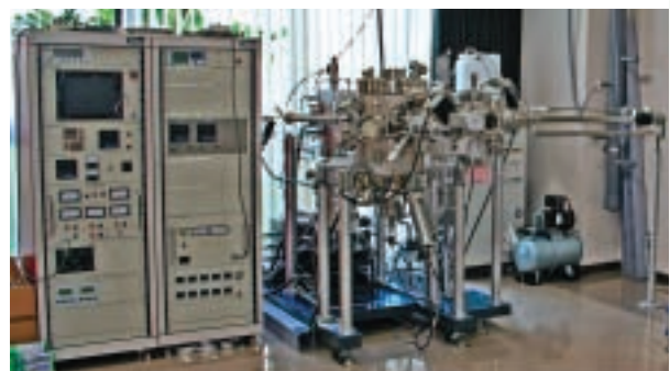
Fig. 1 Molecular beam epitaxy system for thin film and self-organized magnetic arrays installed in Uruma Laboratory.
